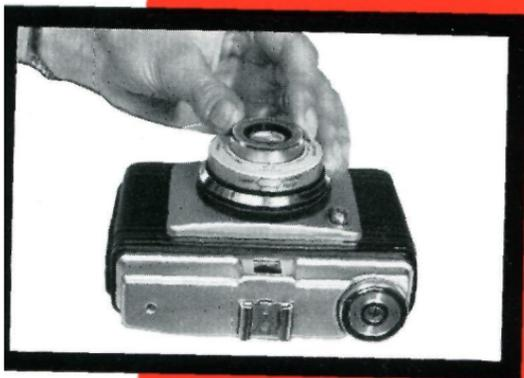
side of the camera, pull up the small knurled stud at the bottom of the chamber, and engage the hole at the end of the spool with the small stud at the bottom. Place the spool in the chamber by pushing back the small knurled stud, then push down the wind-on knob and, holding the spool upright, turn the knob until the slot of the spool engages the wind-on knob.
